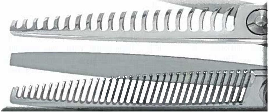
**Wee-Teeth or Serrated Teeth** refers to fine grooves that are cut into the blade surface on the tip of the teeth of a texture shear. These small teeth hold the hair in place when making a cut.
