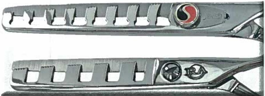
These shears have wider teeth and wider spaces. They typically have from 5 to 9 teeth and cut a significant notch into the hair section. The uncut hair is also in wider pieces so the texture is obvious between the cut and uncut hair. These can be used on many clients but you must expect aggressive texture from these shears.
